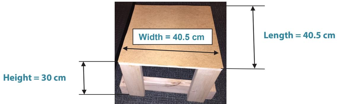
**B)** Your bridge must be able to span a **1 meter gap** between the two **Support Blocks** described above. Your bridge is allowed to rest upon the top surfaces of the **Support Blocks** and should have an overall length of **> 1 m and  $\leq$  1.8 m**. This overall length includes **ANY** supporting bridge components.
